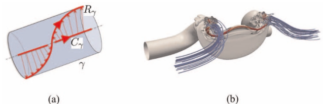
Figure 4 | (a) Flux tube \gamma centered on spatial curve C_\gamma ; (b) vortex lines (blue) and vorticity isosurface (solid grey) under reconnection. (a) The ribbon R_\gamma is formed by connecting C_\gamma with one of the field lines in \gamma . (b) Note the bridge region (threaded by the red line) formed by the reorganization of the weaker vorticity. From a direct numerical simulation of the Navier-Stokes equations 11 .
