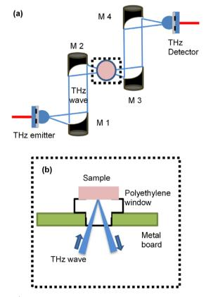
**Figure 5** | (a) A schematic of the experimental setup for the THz wave reflection measurements. (b) Side view of the dotted box in Fig. 5a.
