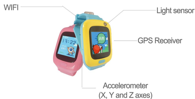
Figure 2. The construction of the smartwatch.
