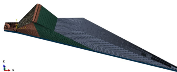
Figure 4. Generalized numerical model of CFRD with pressure slope when the dip angle of the dam foundation is 15°.
