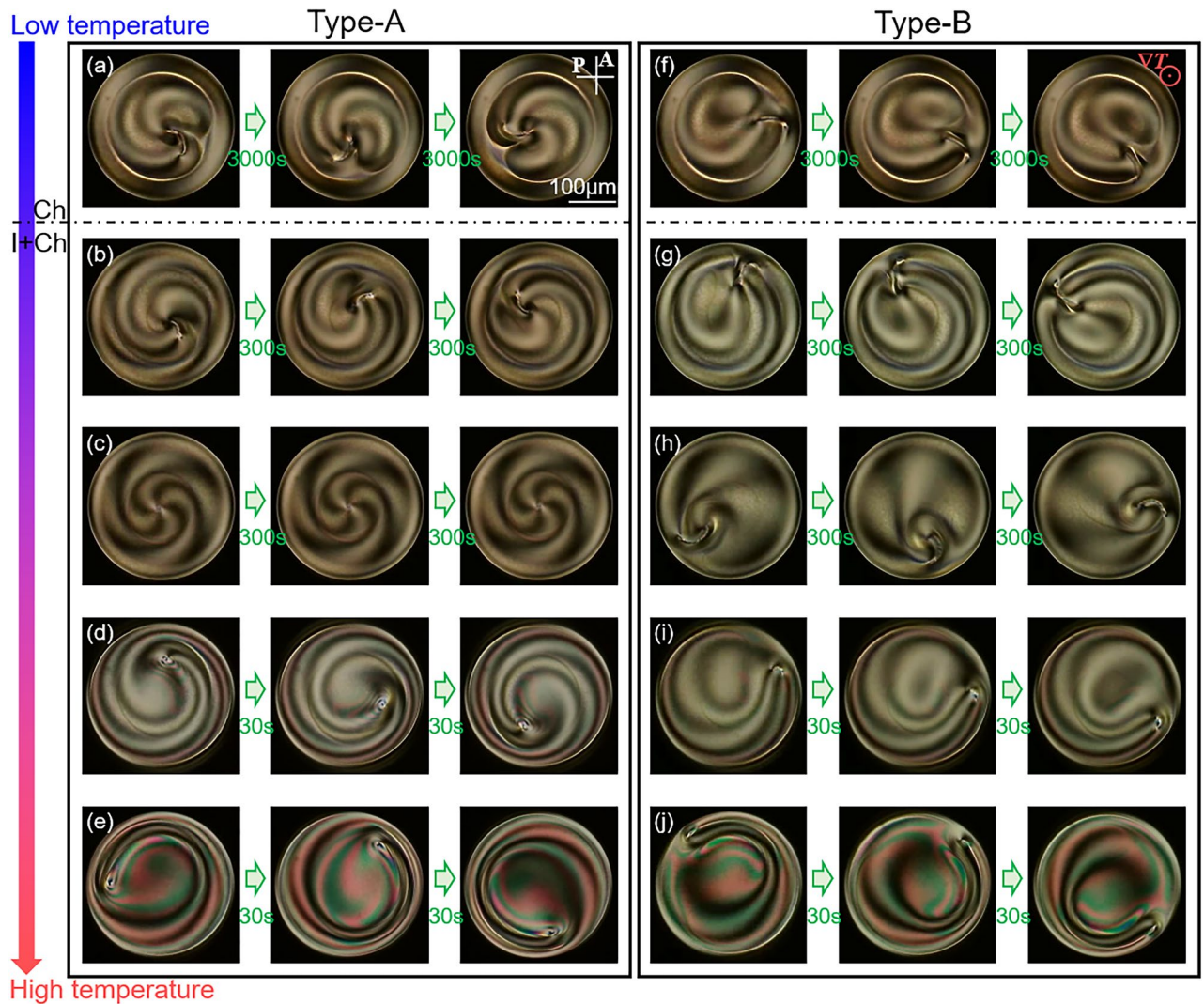
Figure 5. Director rotations under steady states. The time evolutions of POM images are shown. A and P in (a) indicate analyser and polariser respectively, and the white bar 100 \mu\text{m} . Red symbol in (f) indicates the direction of the temperature gradient. \Delta T is set to be 10 K, and T_0 is 35.0 ^{\circ}\text{C} in (a) and (f), 37.5 ^{\circ}\text{C} in (b) and (g), 38.5 ^{\circ}\text{C} in (c) and (h), 42.0 ^{\circ}\text{C} in (d) and (i) and 43.0 ^{\circ}\text{C} in (e) and (j), respectively. (a) and (f) are observed in the Ch phase, and the others are in the I + Ch phase. Time interval in each figure is 3000 s in (a) and (f), 300 s in (b), (c), (g) and (h) and 30 s in (d), (e), (i) and (j). Clockwise rotation was observed in (a), (d)–(f), (i) and (j), while counter-clockwise was in (b), (g) and (h). The corresponding movies are available in Supplementary Video 9.
