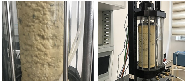
Figure 4. The preparation of samples for the resilient modulus test.
