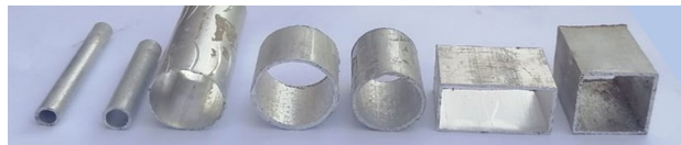
Figure 5. Aluminum 6060 hollow tubes.
