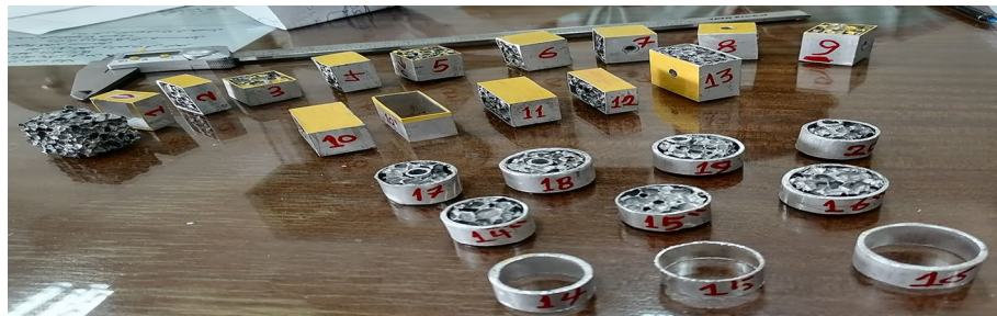
Figure 7. Samples of Aluminium foam Blocks with limited sizes.
