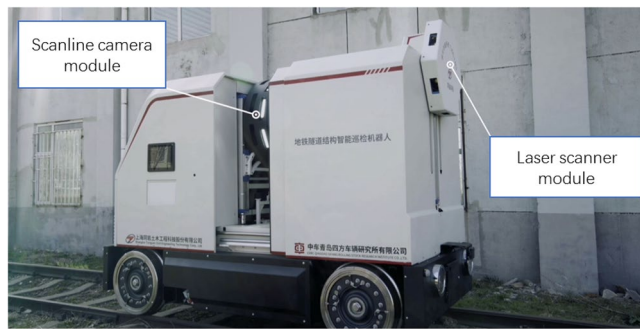
Figure 6. Tunnel inspection robot.
