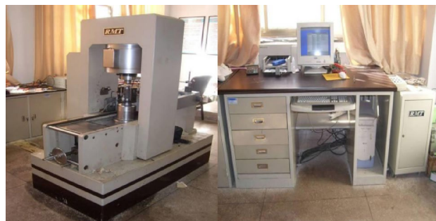
Figure 9. Rock mechanics test system and acoustic emission system.
