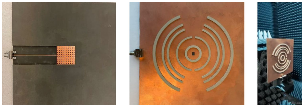
Figure 23. Fabricated Prototype, bottom (left), top (middle), and right (isometric view).
