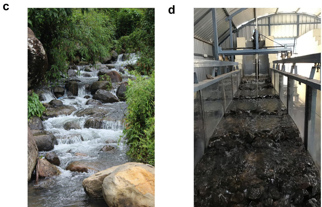
Figure 1. Details of step-pool systems in the present study: (a) Longitudinal section of the field site, (b) Longitudinal section of the laboratory model, (c) Photograph of the field site, (d) Photograph of the experimental setup.
