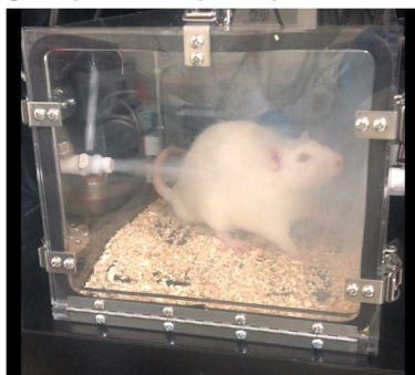
Figure 1. Vapor delivery system. (A) Illustration of passive vapor delivery system: Schematic of vapor apparatus components with direction of air-flow (adapted from Freels et al. 5 ). Briefly, the vapor inhalation system uses machinery similar to electronic cigarettes to deliver distinct “puffs” of vapor within airtight chambers. A vacuum compressor pulls ambient room air through an intake valve at a constant rate of 1 L per minute. At set intervals THC-dominant cannabis extract is vaporized combining with the constant ambient air flow for delivery into the chamber. Air (and vapor) are evacuated through the back of the chamber via the vacuum compressor, filtered and ventilated out of the building. (B) Image of passive vapor exposure: Picture of a male SD rat within the vapor apparatus.
