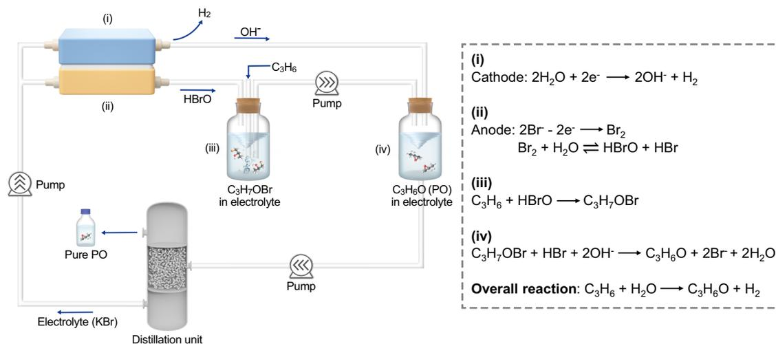
**Fig. 1 | Schematic illustration of the electrochemical bromohydrin route for efficient synthesis of PO.** Propylene was first converted to C<sub>3</sub>H<sub>7</sub>OBr in an independent reactor through a bromide mediator; this product was then mixed with
