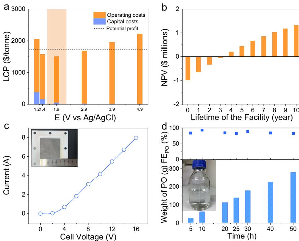
**Fig. 3 | TEA and large-scale production of PO. a** LCP of the electrochemical bromohydrin route at different applied potentials. **b** End-of-life NPV values of the electrochemical bromohydrin route at  $250 \text{ mA cm}^{-2}$ . **c** The steady-state current of the enlarged electrode with a geometric area of  $5 \times 5 \text{ cm}^2$  in  $0.4 \text{ M KBr}$ . The inset
