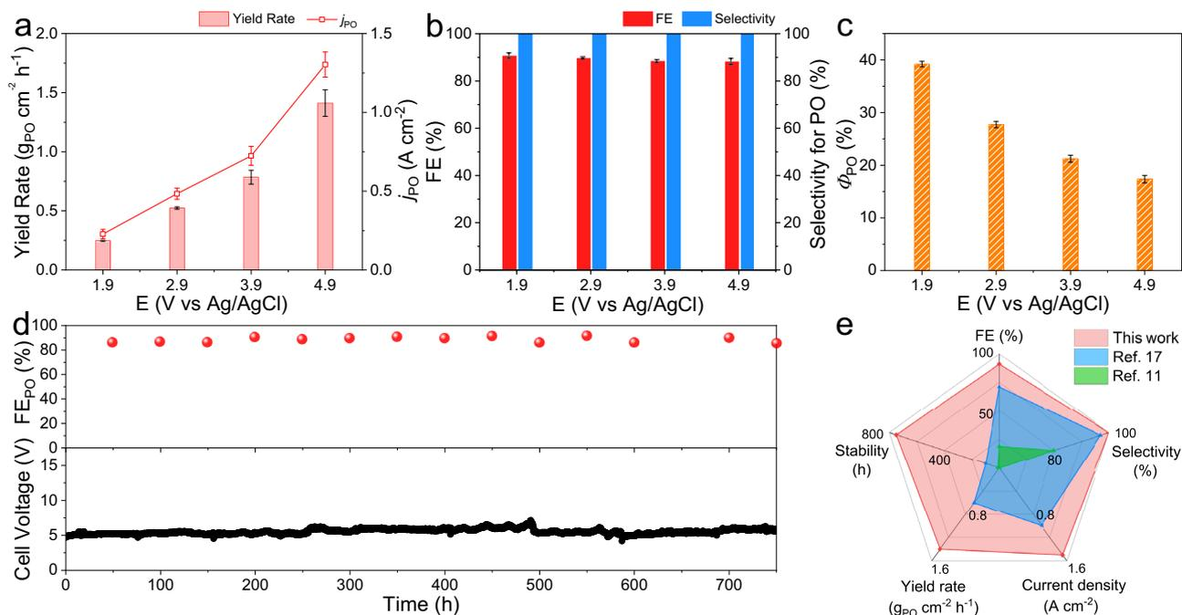
**Fig. 2 | Catalytic performance and long-term stability of the system.** a–c  $j_{PO}$  and yield rate for PO (a),  $FE_{PO}$  and selectivity for PO (b), and  $\Phi_{PO}$  (c) at different applied potentials. d Stability test during 750-h (>30 days) continuous electrolysis at a constant current density of  $250 mA cm^{-2}$ . e Comparison of FE, current density,
