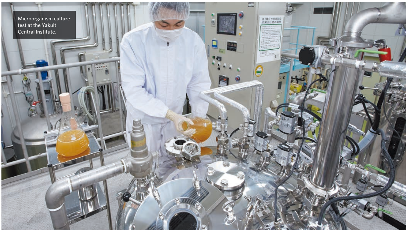
Jar fermenters at microbial culture testing stations at the Yakult Central Institute.
