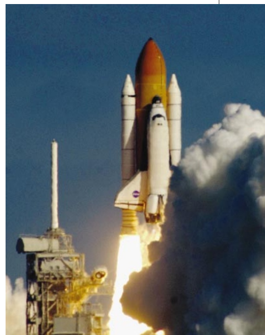
Crumbling foam from the nose of Columbia's launcher (orange) may have damaged the craft.
