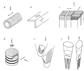
orientations. f, Suggestion of Cameron and Pugh<sup>1</sup> for the sunfish: the cone inner segments act as elliptical wave-guide polarizers, conveying selectivity on the double cones beneath. Open arrows indicate light direction and thin arrows the plane of polarization selectivity.
