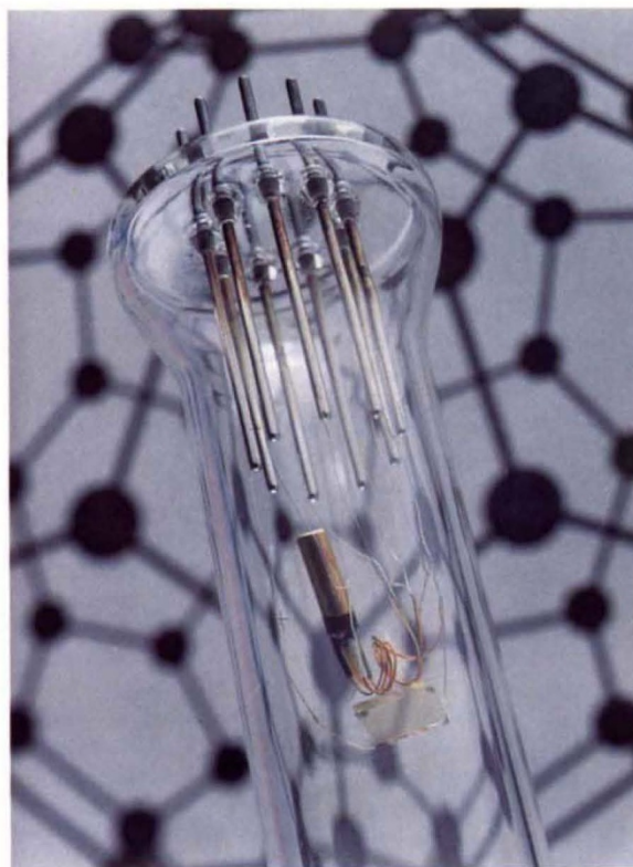
FIG. 2 The apparatus of Hebard et al. The superconducting doped C_{60} film is on the glass square near the bottom. The sealed tube contains inert helium to protect the fragile film.
