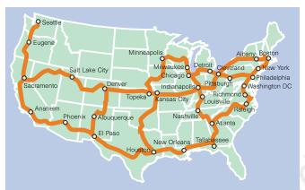
Hot wired: the new Abilene network will form a high-speed data communication backbone serving the main research universities in the United States. Fibreoptic cables will run mainly under railway lines, where they will be relatively safe from accidental disruption.
