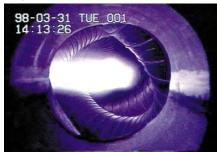
[TOKYO] Scientists at Japan's National Institute of Fusion Sciences witnessed the successful first operation of the world's largest stellarator fusion device last week. The Large Helical Device (LHD), which is designed to explore new aspects of steady-state plasma physics, produced the first plasma (pictured) at 1.5 tesla, which is less than half its maximum magnetic energy. The institute aims to bring the reactor up to its maximum capacity over the next six months.
