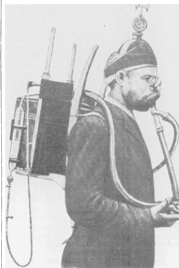
Deep breathing — the first portable respirometer, designed by Zuntz and co-workers in 1906. The open-circuit apparatus made possible the long-term measurement of energy expenditure during a range of activities. The equipment consisted of a mask with manually-operated taps, a dry gasmeter and a mercury tonometer for collection of expired air samples, and was the forerunner of the Max Planck respirometer. The picture is taken from Animal and Human Calorimetry by J. A. McLean and G. Tobin, a survey of the theory and techniques of calorimetry as applied to the study of energy metabolism in humans and animals. The book is just published by Cambridge University Press and costs £37.50, $69.50.
