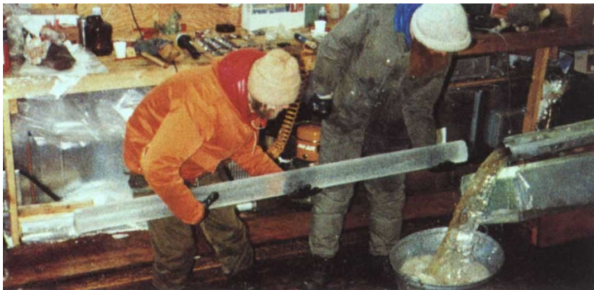
Removing an ice-core sample that dates back approximately 50,000 years to the glacial period.
