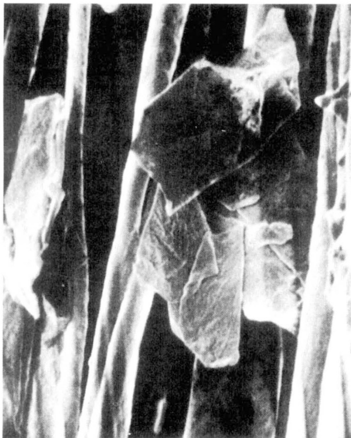
Epithelial cells adhering to the collar of a cotton-polyester shirt as seen under the scanning electron microscope. The photograph is reproduced by courtesy of 'Stereoscan', Kent Cambridge Scientific, Inc., in Detergency , part 1 of volume 5 of the surfactant science series, edited by W. G. Cutler and R. C. Davis (Marcel Dekker, New York, 1972).
