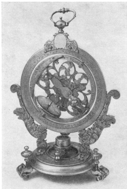
Mechanical equinoctial dial by Wm. Deane of London, c. 1690 (from Sundials , by F. W. Cousins, p. 65). (Photo by courtesy of the National Maritime Museum.)
