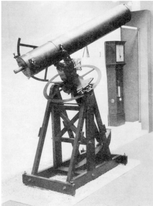
A 49 inch focus, 9¼ inch aperture Gregorian reflector, made by James Short for the Paris Observatory, which lent it to the Royal Scottish Museum for the exhibition.
