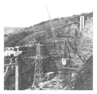
towers through steel wires attached to two rams in the side of the quarry—one can be seen in the picture—and hydraulic rams anchored to the floor. A variety of different tests can be carried out, leading ultimately to a test to destruction which reveals whether or not the structure fulfils specification. The picture shows a new type of 400 kV tower being tested for the CEGB which is only 100 feet high, compared with the 165 feet of the usual 400 kV tower.
