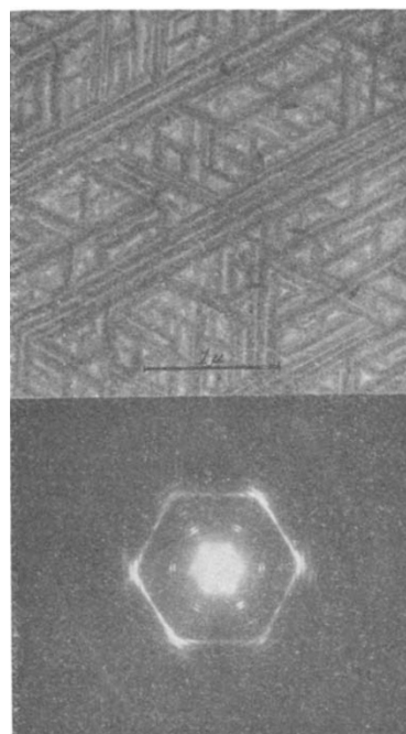
Fig. 1. Vacuum-evaporated film of platinum phthalocyanine on muscovite
