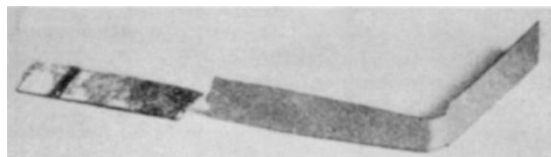
Fig. 1. Strip of zirconium with 6 at. per cent oxygen, after gradient-heating. The thinnest part is ductile and bent, the thick parts remain brittle and one end is broken
