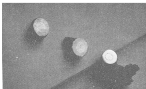
Fig. 2. Cross-sections of 'slugs' showing the copper cores
