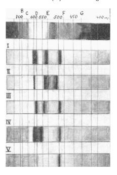
pigment shows no absorption maxima in the visible range, but an extinction of colour in the violet and red regions of the spectrum. Unfortunately, because of its very low concentration, we could not distinguish absorption bands.
