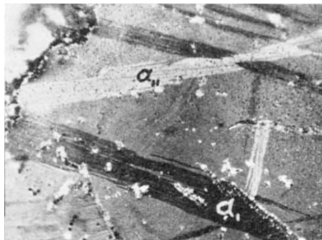
Fig. 1. Plates of \alpha -phase formed in a \beta -crystal. The plates examined are marked \alpha , and \alpha_n . Polarized light. \times 150
