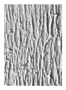
essentially fibrillar character. The diameters of the fibrils appear to lie between about 200 A. and 1000 A., and there are several of the larger fibrils which seem to be built up of those of diameter about 200 A. This suggests that the 200-A. fibrils might be the fundamental ones, and also that there might be an upper limit, indicated by the 1000-A. fibrils, to the extent to which the fundamental fibrils can conveniently group together.
