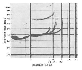
An experiment carried out at Fort Chimo (lat. 58.1° N., long. 68.3° W.) on September 30, 1950, showed the polarization of the Z-trace to be ordinary. or in the northern hemisphere, anticlockwise as viewed in the direction of propagation. This is compatible with the theory that the Z-trace is the longitudinal ordinary reflexion (made possible at off longitudinal directions by the effect of collision<sup>2</sup>), rather than an earlier view that it is the second extraordinary reflexion.
