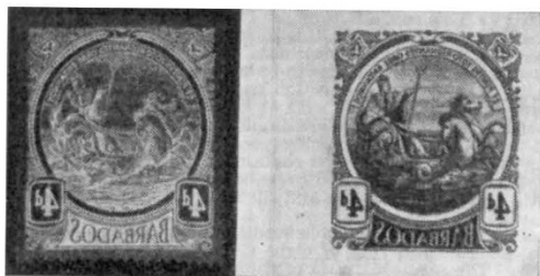
(a) Radiograph with 10 kV. X-rays; (b) 'radiograph' with 190 kV. X-rays.
