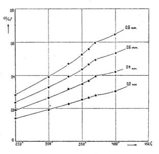
Chevenard<sup>1</sup> and Williams<sup>2</sup> found also by means of measurements on the thermal expansion coefficient of nickel some discontinuities at the Curie point. These discontinuities are, however, too small to explain the phenomena observed by us. It is known that activated adsorption is connected with the electronic state of the metal, and at the Curie point this state undergoes some characteristic modifica-
