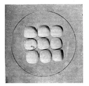
shape. The samples shown in the reproduction at approximately actual size were originally essentially spherical and assumed this dice-like shape after a few months of service. Their original size was approximately twice that shown. The manufacturers of these balls state that they are made by extruding a cylindrical column of batch, cutting this off into lengths, and rolling to give sphericity. Had the extruded section been square an obvious explanation would have suggested itself.
