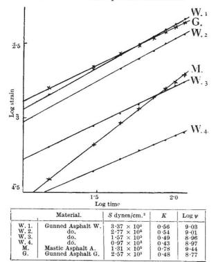
If the extension (and recovery) is plotted against time, curves are obtained which indicate that there is little or no immediate elastic extension on applying the load, or recovery on removing it, but the extension portion of the curve may be regarded as an elastic
