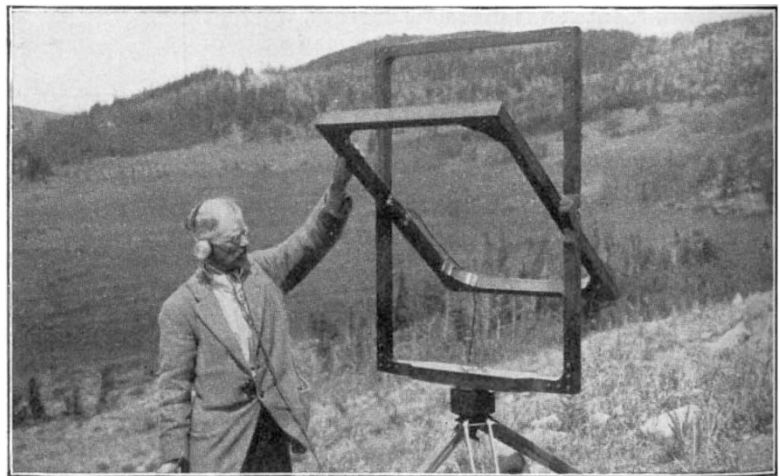
FIG. 3.—Transit tripod with coil, turning in azimuth or dip, and the telephones. Large horizontal loop with 500-cycle alternating current. Near Caribou Mine, Colorado.
