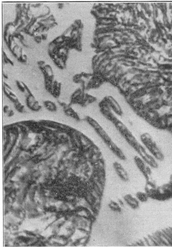
FIG. 1.—Phosphide eutectic in cast iron. \times 5000 .
