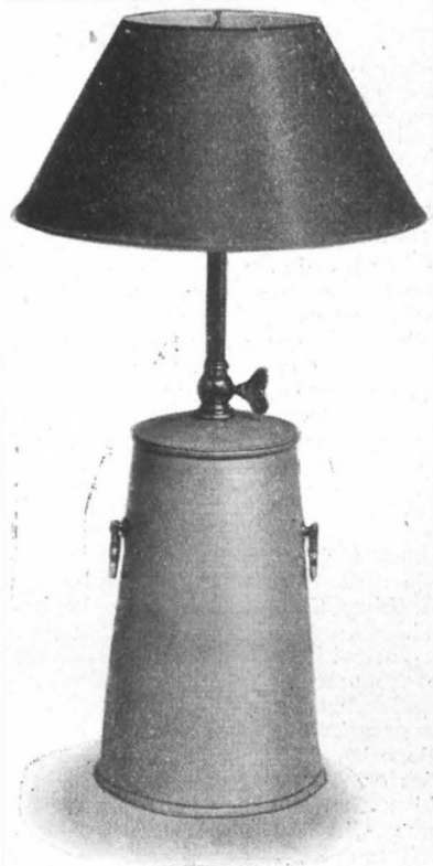
FIG. 3.—Portable acetylene lamp of very simple construction; requires 1 lb. of carbide and is stated to give 50 candle-power for eight hours.
