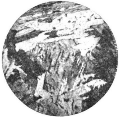
FIG. 4.—Swedish Iron heated to the point of Incipient Fusion (Osmond, "Sur la Cristallographie du Fer"). Magnified 16 diameters.
