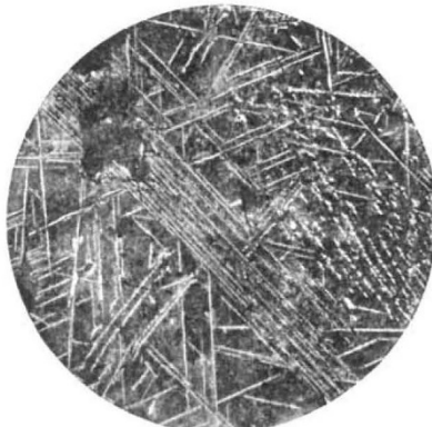
FIG. 6.—Widmanstätten Structure in Alloy of 90 per cent. Platinum and 10 per cent. Aluminium (Chouriquine, "Sur les alliages du Platine avec l'Aluminium"). Magnified 50 diameters and slightly reduced.
