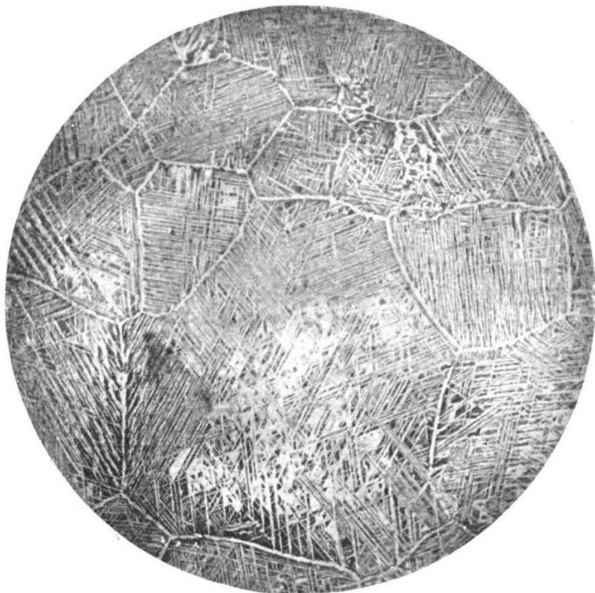
FIG. 1.—Widmanstätten Structure in Carbon Steel (Carbon 0.55 per cent.). Alloy No. 8. Magnified 8 diameters.
