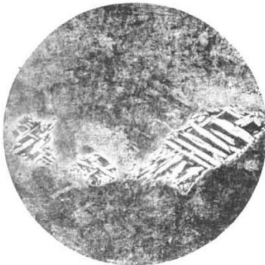
FIG. 5.—Widmanstätten Structure in Bronze, containing 55.1 per cent. Copper. Cooled in Sand and Annealed (L. Guillet, "Les Laitons au Nickel"). Magnified 30 diameters and slightly reduced.
