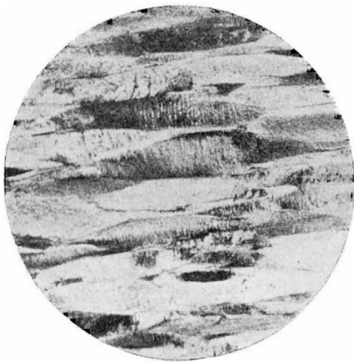
FIG. 1.—Structure of pure gold after being rolled, \times 11 .
