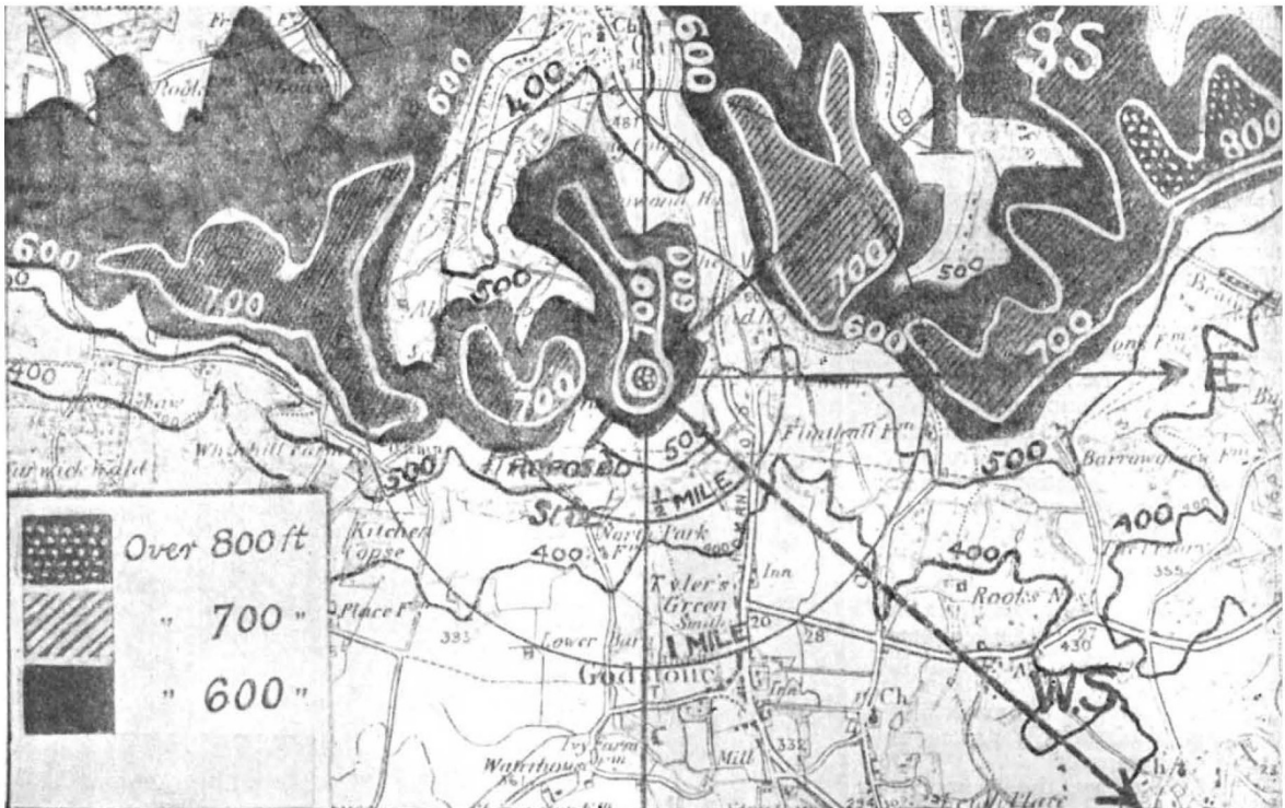
FIG. 2.—Fosterdown. The selected site, 600 feet above sea-level, is at the centre of the half-mile and mile circles, and lies 100 feet above all the neighbouring country with the exception of the small 800-foot area to the north of east, which is on the same level as the site. The lines SS and WS are the directions of sunrise at the summer and winter solstices. The figure shows the open and clear nature of the horizon in all directions.
