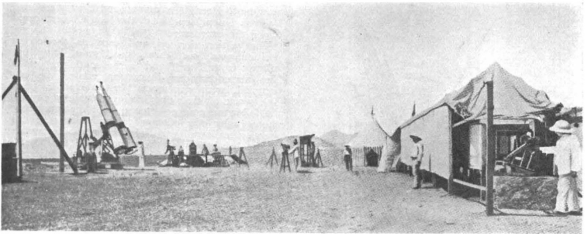
FIG. 1.—The Hamburg Observatory's Eclipse Camp in Souk-Ahras. The 20-metre coronagraph is on the right, and the twin equatorial planet-finder on the left.
