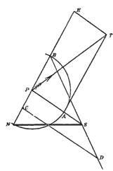
duced, so that PA = PB = PN. Take C in BN, so that BC measured towards N equals PS. Draw CD parallel to PS, D being in the line BS. Measure PE away from N, so that PE = CD. The diagonal PT of the paral-lelogram AE is the direction required.
