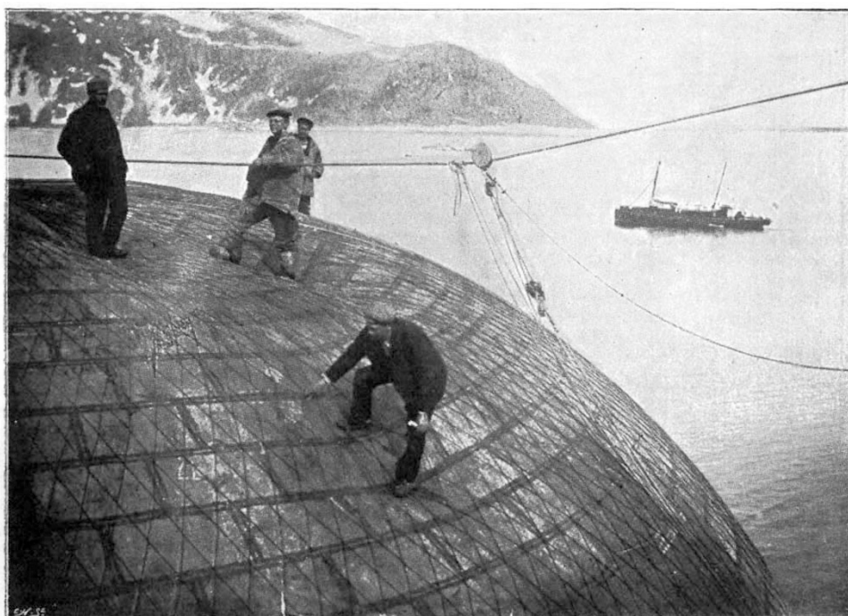
FIG. 1.—The top of the balloon, showing the joinings of the pieces.
