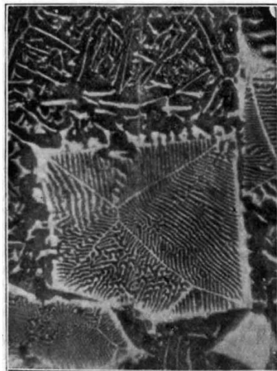
FIG. 2.—Magnolia metal. Magnified 200 diameters. Pb, 80 per cent.; Sb, 15 per cent.; Sn, 5 per cent.
