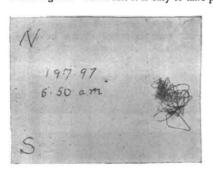
sensitised sensitised paper, and I send you some of the results [one of the prints is here reproduced] I have already obtained. The trace is magnified 6.7 times by the instrument, so that one can form an idea from it of how exceedingly minute the actual movement of the surface is, and yet
