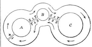
battery to these borders. By aid of movable electrodes of a voltmeter trace, on the metallic surface, and a very large number (n-1), of equidifferent equipotential closed curves between the + and - borders. Divide any one of these equipotentials  $^2$  into parts each equal to the
