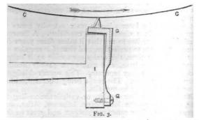
should the striker, T, be still kept raised, the pricker will rest upon it, but its point will be free of the cylinder, and at some distance, D, below it. The strikers,  $T_{11}$ , &c., are worked by electro-magnets : the spiral spring shown just above the head of each pricker, is compressed when the pricker is projected between the head and sheath, and assists in the disengagement of the pricker from the paper. The punctures of the prickers are very marked and distinct.
