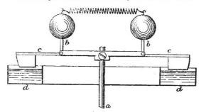
As the balls go out a component of their weight comes into action, helping this motion and opposed to the pull of the spring. For small displacements this force increases very nearly in proportion to the displacement, and hence, by choosing a spring of suitable stiffness, a small change of speed can be made to produce a relatively very large displacement, the proper condition for approximate isochronism.
